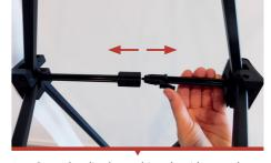
2. Open the clips by pushing the sides, a red safety mark will appear
